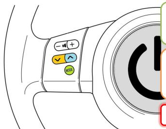
In **mixed control mode**, the user can activate any connected camera with OEM steering wheel controls. For this purpose three buttons are used: **MODE**, **SEEK+**, **SEEK-**. Below are the control algorithms (choosing different modes) with OEM steering wheel controls.
